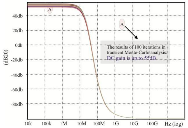
Fig.7 DC gain of the proposed VGA by applying 2%variation of the transistors threshold voltage
