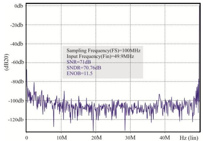
Fig.8 Output FFT spectrum of the proposed VGA
