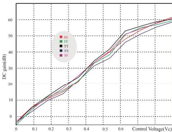
Fig.5 DC gain vs. the Control voltage (Vc) in all corners
