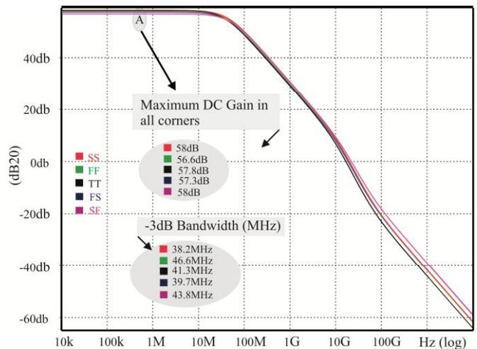
Fig.2 Ac simulation for maximum gain in all corners
