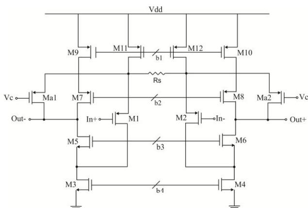
Fig.1 The proposed VGA circuit
