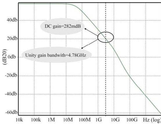
Fig.4 Unity gain bandwidth of the amplifier in TT corner
