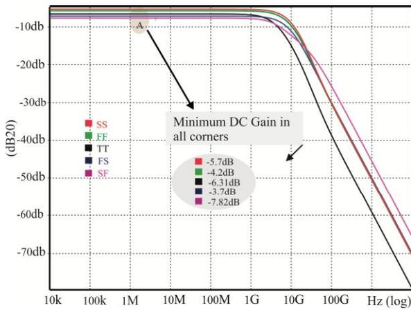
Fig.3 Ac simulation for minimum gain in all corners
