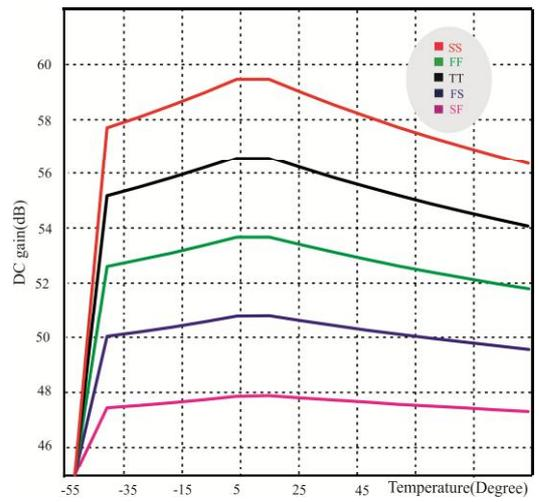
Fig.6 DC gain vs. Temperature in all corners
