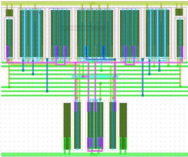
Fig.9 Layout of the proposed VGA
