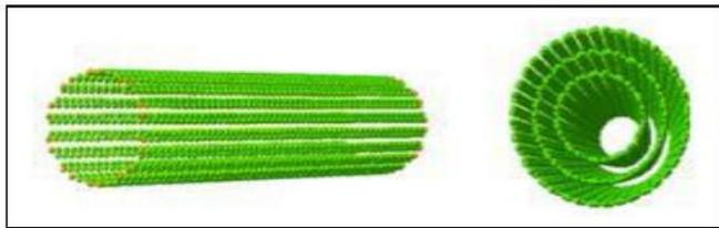
Figure 1. Single walled and multi walled nanotubes[5].
