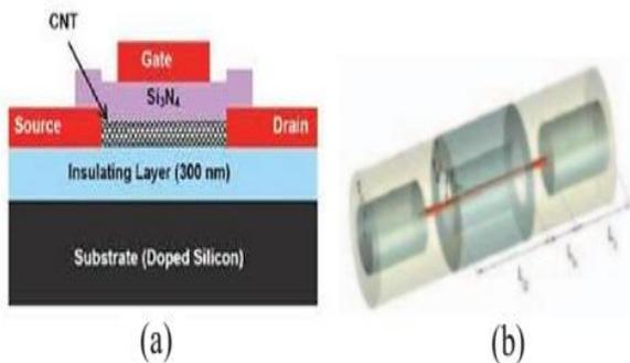
Figure 4. Geometry of CNTFET (a) planar (b) coaxial[9].
