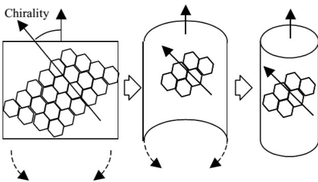
Figure 3. Chirality of a CNT [6].
