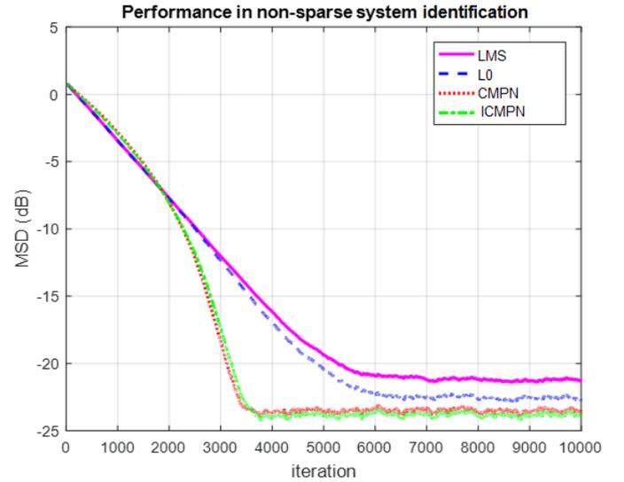
Fig. 4. The identification of a system with 256 non-zero taps.
