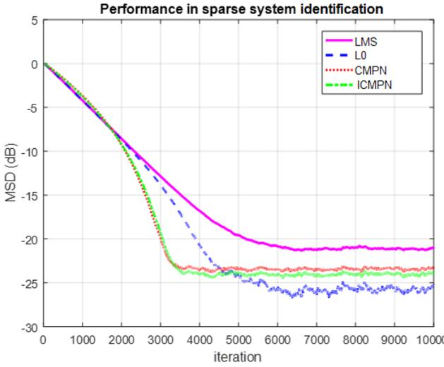
Fig. 2. The identification of a system with 256 taps and only 28 non-zero elements.
